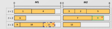
Fig. 5. \mathcal{N}_4 – Exchange between two jobs from the same period, but from different machines, and an insertion of another job in the considered period. Solution S' \in \mathcal{N}_4(S) .
