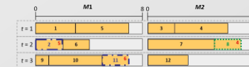
Fig. 6. \mathcal{N}_5 – Exchange between two jobs from necessarily adjacent periods. Solution S' \in \mathcal{N}_5(S) .
