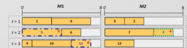
Fig. 7. \mathcal{N}_6 – Exchange between two jobs, from the same period, but from different machines. Solution S' \in \mathcal{N}_6(S) .
