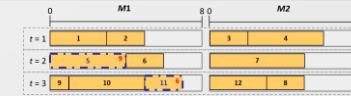
Fig. 2. \mathcal{N}_1 – Insertion of one job in another period. Solution S' \in \mathcal{N}_1(S) .
