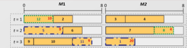
Fig. 3. \mathcal{N}_2 – Exchange between two jobs from different periods. Solution S' \in \mathcal{N}_2(S) .
